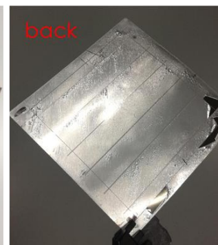
Figure 11. Photos of the flexible minimodule before and after removal from the glass carrier.
